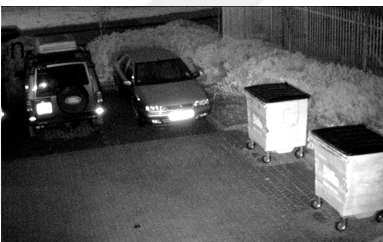
Night time – IR On High Sensitivity infrared response with varifocal lens.
